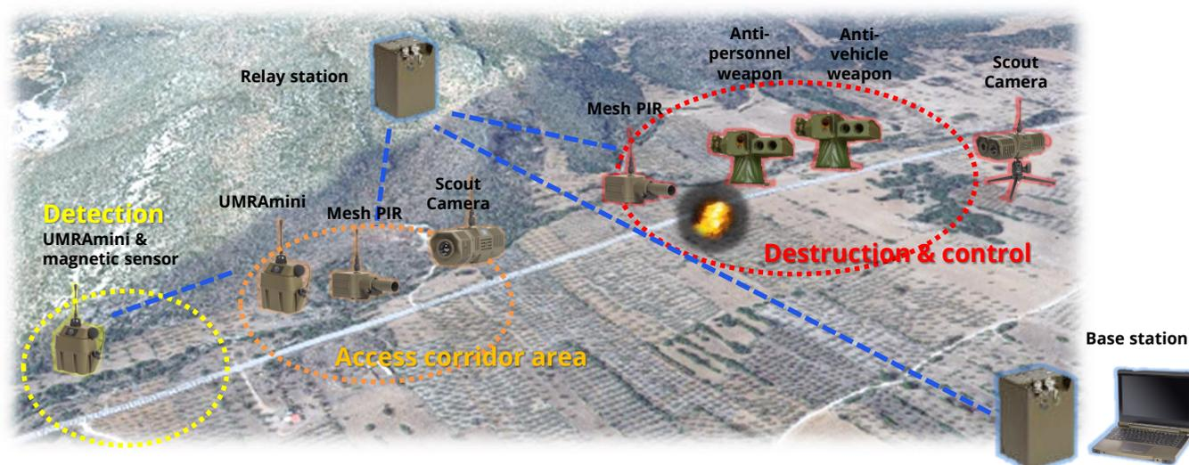
1. If a moving object is approaching the access corridor, the UMRAmiri seismic & acoustic sensor in conjunction with a magnetic sensor will classify the threat and give an early warning to the operator positioned at the Base station.
